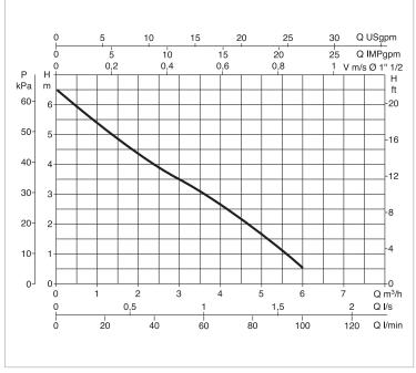
$\label{thm:continuous} The performance curves are based on kinematic viscosity values = 1 \ \text{mm}^2/\text{s} \ \text{and} \ \text{density} \ \text{equal} \ \text{to} \ 1000 \ \text{kg/m}^3. \ \text{Curve} \ \text{tolerance} \ \text{according} \ \text{to} \ 150 \ 9906.$
